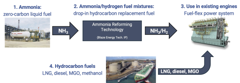
BLAZE SOLUTION: FLEX-FUEL MARINE PROPULSION SYSTEM Solving alternative fuel flexibility challenge through fuel reforming
